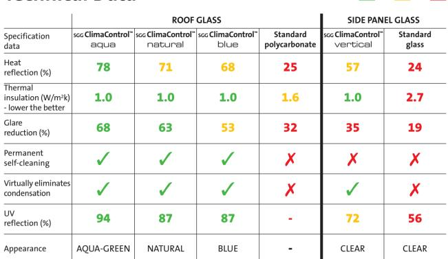
Heat reflection: measured by the taking the opposite or inverse of the glazing solar factor. Solar Factor is the percentage of the total solar radiant heat energy entering the room through the glass.
