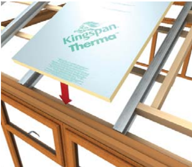
Install external insulation
